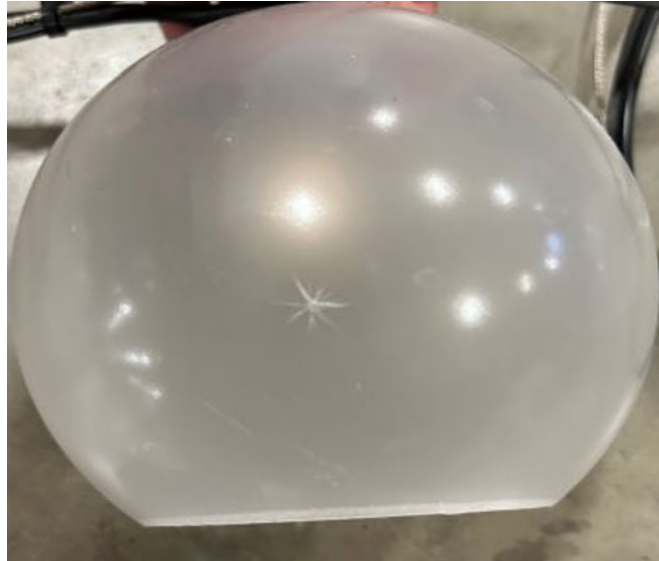
Photos showing cracks on the bulbs from impact
