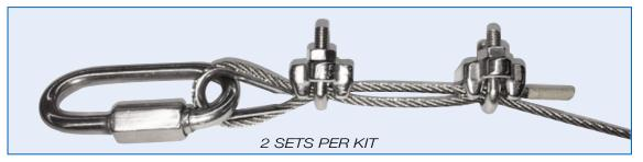
Stainless Steel Termination Hardware Kit for most suspensions installed with a catenary droop. Working system load, 175#. Includes quick link for easy installation and servicing. Kit includes terminations for both ends c/o:
