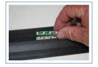
PLACE NEW LED CIRCUIT BOARD BACK ONTO THE TWO BRASS PINS
