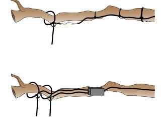
12 VAC systems require remote class II transformer mounted at base of tree.For security, best to stub up into tree using rigid or seal tight flex
