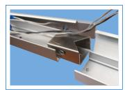
Insert flex joiner in to the pre-attached screw on to the next section, connect and secure using the provided flat washer and nylock nut. A 5/16" nut driver is the correct tool.
